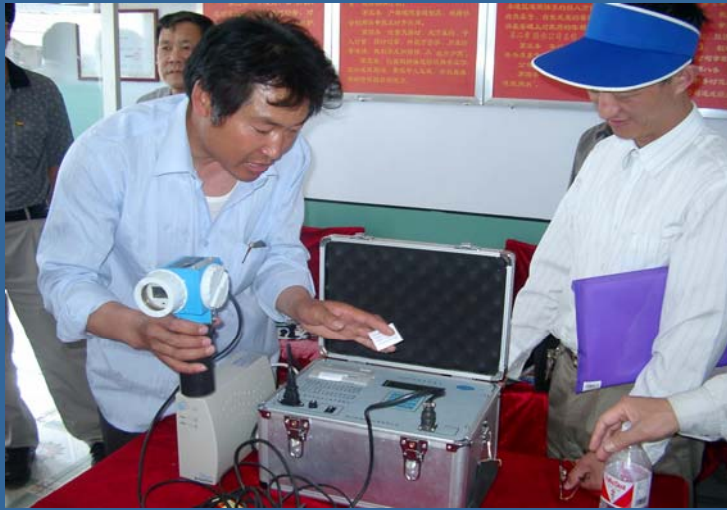
Manager of Zunhua WSC in Hebei explaining portable sonic water measuring device used by WSC to measure water deliveries to WUA clients.
