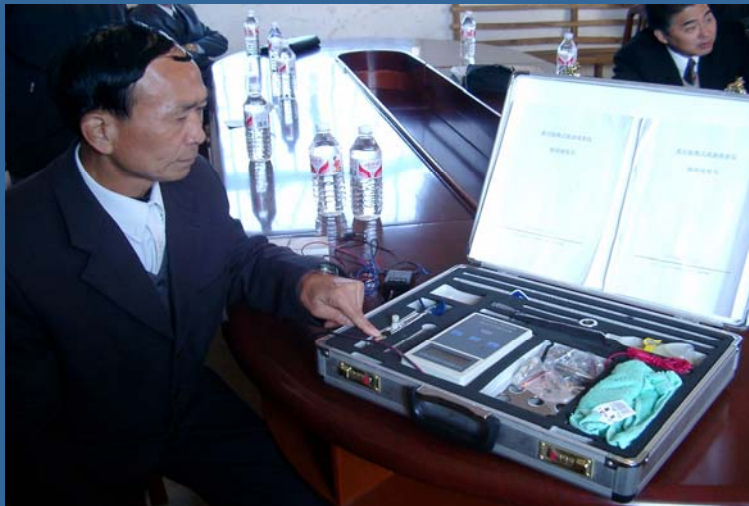
WUA Chairman in Anhui explaining velocity meter used by WUA to measure water deliveries.
